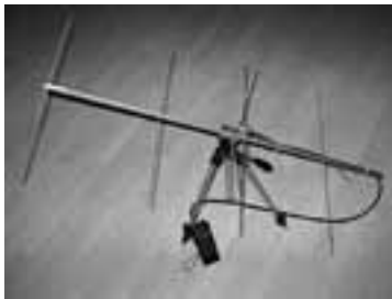
Fig. 1: A 4 elements yagi antenna for 260mhz UHF Military band
